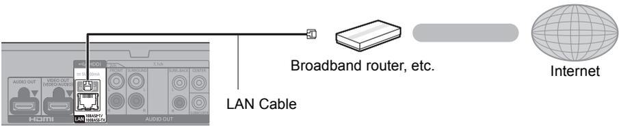
Use category 5 or above straight LAN cables (STP) when connecting to peripheral devices.
